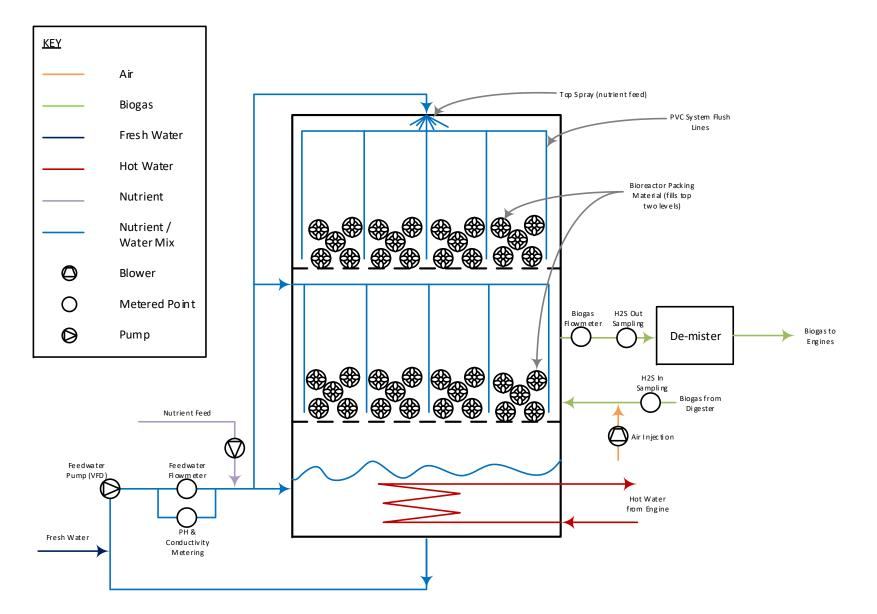
Figure 3. Schematic of New H<sub>2</sub>S Scrubber
