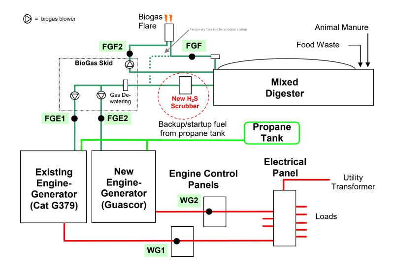
Figure 2. Schematic of ADG System
