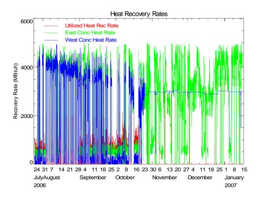
Similar to the heat recovery rates, the cogen gas flow data is inconsistent. The gas flow rates for generator 2 shows many periods of repeating data beginning in October. The Total Cogen Gas Flow data appears to be the simple sum of the two CG Flow Meters, and thus includes the repeating data.
