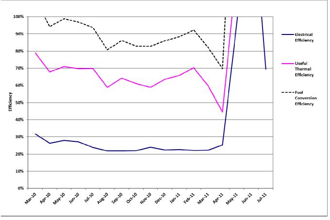
FIGURE 5 CHP SYSTEM EFFICIENCY BY MONTH
