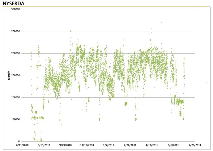
FIGURE 7 CHP USEFUL THERMAL OUTPUT VERSUS TIME
