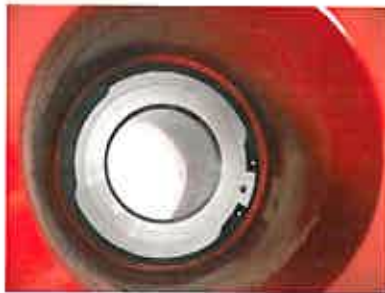
DN100 with orifice plate 3
